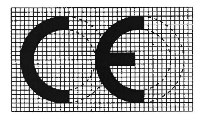
If the 'CE' conformity marking is reduced or enlarged the proportions given in the above graduated drawing must be respected.
